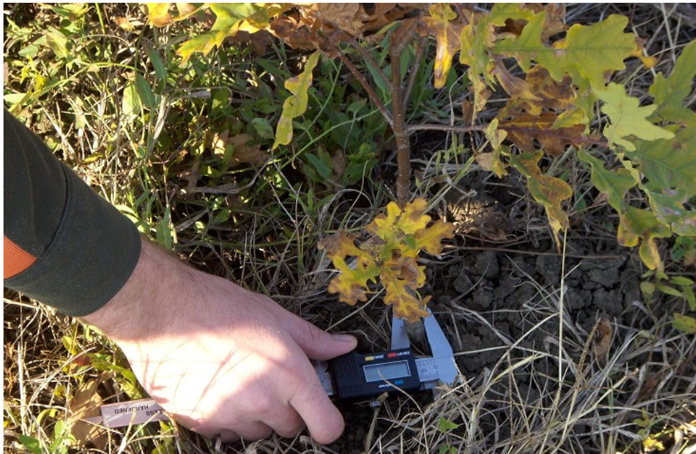
Measuring the diameter with electronic callipers
